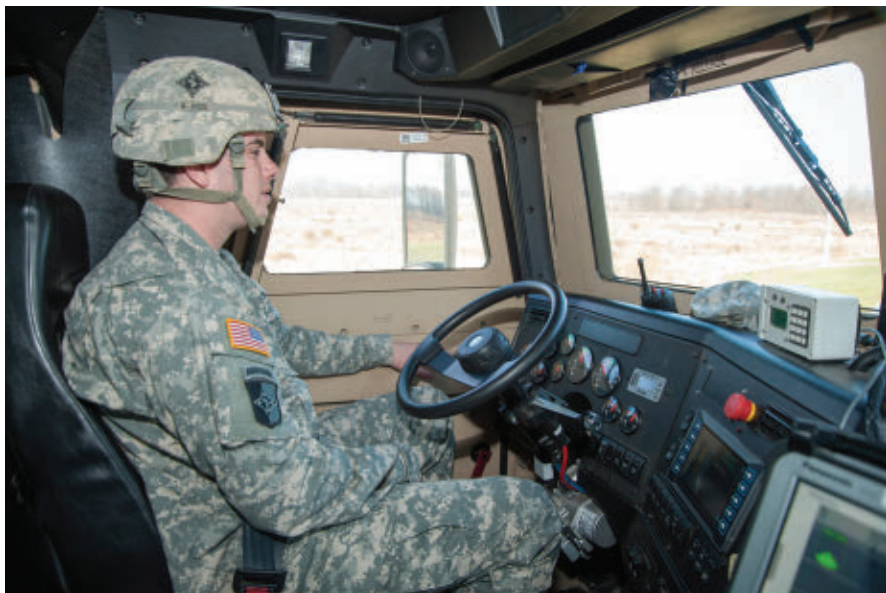
The U.S. Army military line-haul tractor with the Autonomous Mobility Appliqué System offers driver-assist or autonomous features like leader-follower.
