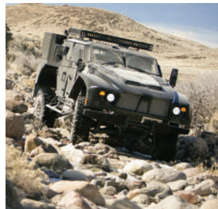
This vehicle is a demonstrator for the Light Combat Tactical Vehicle (LCTV), which will have optionally driven capabilities.
